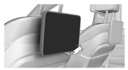
Pull on the bottom edge, see arrow, or press the lower edge in order to adjust the tilt.
