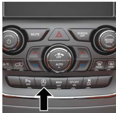
STOP/START Off Switch
