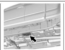
The fuel filter is on the driver side, inside the frame rail in front of the fuel tank.
