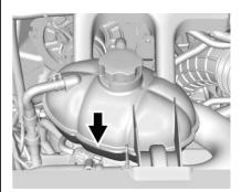
The coolant surge tank is near the center of the engine compartment. See *Engine Compartment Overview* ⇒ 86 for location.
