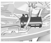
If equipped, the FOH will enhance heater performance and will reduce the amount of time it takes to warm the inside of the vehicle in cold conditions below or equal to 4 °C (39 °F).
