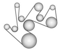
6.6L 8-Cylinder Engine (L5P Dual Generator)
