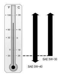
Cold Temperature Operation: In an area of extreme cold, where the temperature falls below -29 °C (-20 °F), an SAE 0W-40 oil may be used. An oil of this viscosity grade
