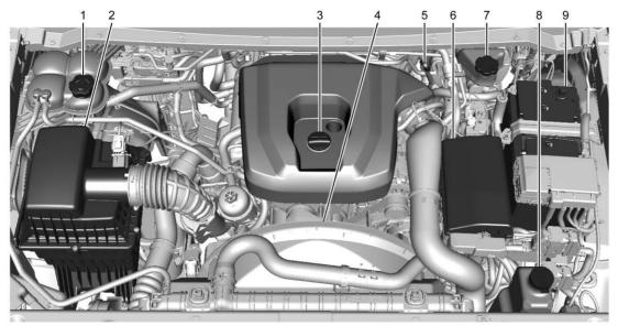
2.8L 4-Cylinder Engine Pickup Models
