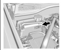
The coolant surge tank is divided into two sides. The upper should be filled to the indicated mark. The lower portion will be mostly empty, depending on the operating temperature.
