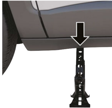
Front Jacking Location
