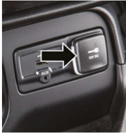
Front Power Outlet
