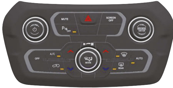
Automatic Temperature Controls (ATC)
