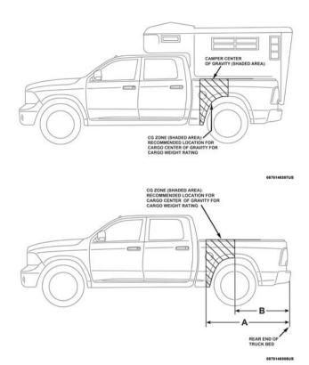
The tables on the following pages designate the Cargo Weight Rating and the Center of Gravity Zone for each vehicle listed.
